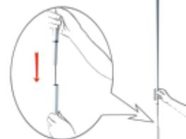
9. Take the support pole link up to a whole pole along the direction of the elastic.
