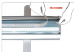
5. Tear out the adhesive tape from the PVC sheet.
