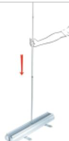
10. Insert the support pole into the hole on the base.
